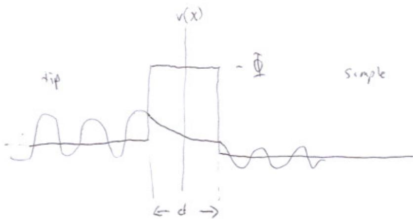
electron can tunnel through barrier
