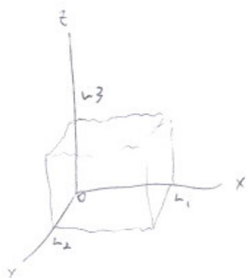
$$\psi(x, y, z) = A \sin\left(\frac{n_1 \pi x}{L_1}\right) \sin\left(\frac{n_2 \pi y}{L_2}\right) \sin\left(\frac{n_3 \pi z}{L_3}\right)$$
