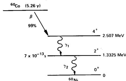
Fig. 3.9. The Decay Scheme of <sup>60</sup>Co.
