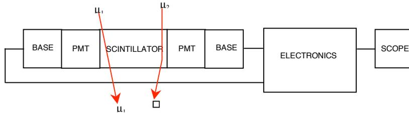
Fig. 1. Schematic setup for muon lifetime experiment.  $\mu_1$  passes through the scintillator losing some energy: A single voltage pulse appears on the scope.  $\mu_2$  stops in the scintillator and decays after time  $t$  to an electron: Two voltage pulses appear on the scope.
