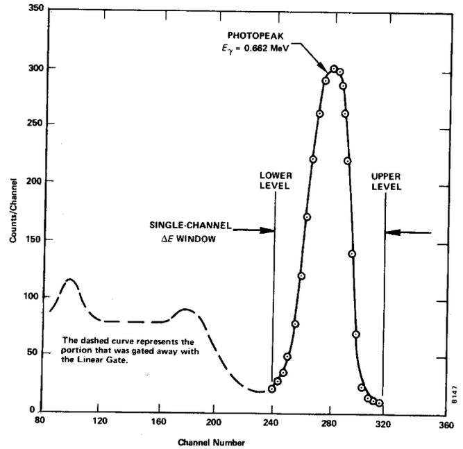
Fig. 3.8.  $^{137}\text{Cs}$  Spectrum with the Linear Gate.
