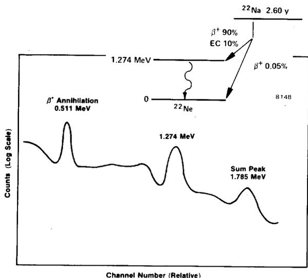
Fig. 3.10. Sum Peak for the <sup>22</sup>Na Source from Source Kit SK-1G.
