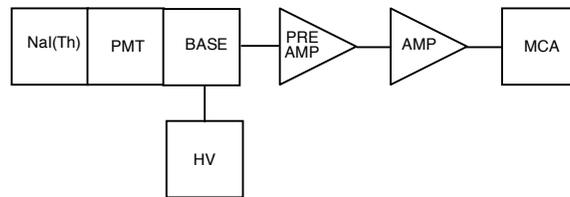
Fig. 1: Schematic drawing of the electronics for  $\gamma$ -ray spectroscopy. The NaI(Th) scintillator crystal, PMT, and PMT Base are a single unit. The high voltage applied to the base is negative and less than 1500 V. The preamp and amplifier are typically Nuclear Instrumentation Modules (NIM) powered by a NIM crate. The MCA is a special purpose electronics plug-in board in a PC.
