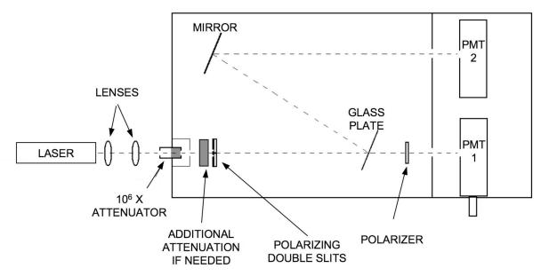
Figure 2. Schematic showing photon coincidence measurement
